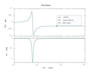
It is observed that the deduced transfer function  $G_{vd}(s)$  is approximately equivalent to that provided online since the result has a gain of 0 dB (gain of 1) and a phase shift of  $0^{\circ}$ , indicating that the deduced  $G_{vd}(s)$  holds true.
